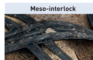
Meso-interlock Interlock between soil particles and geogrid ribs due to surface texture.
