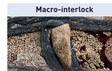
Macro-interlock Penetration of stones and gravel through mesh openings, i.e. full interlock between rock components and grid.
