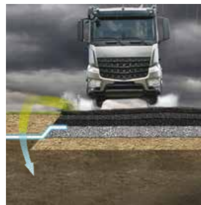
Decentralized precipitation treatment on roads
