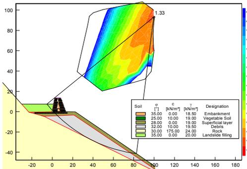
Figure 6. Example of overall stability calculation
