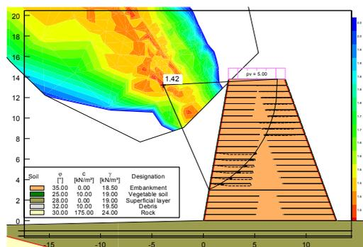
Figure 5. Example of internal stability calculation (back side)
