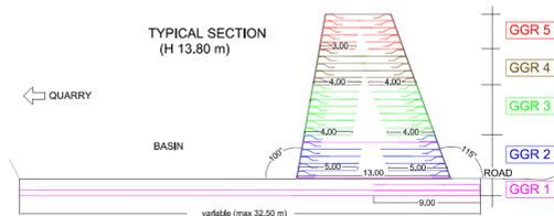
Figure 3. Structural configuration of the embankment
