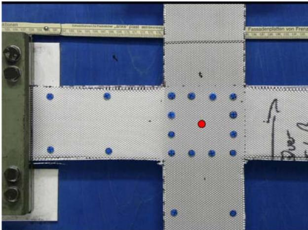
**Figure 2.** Biaxial testing of a woven geotextile at RWTH Aachen, begin of loading
