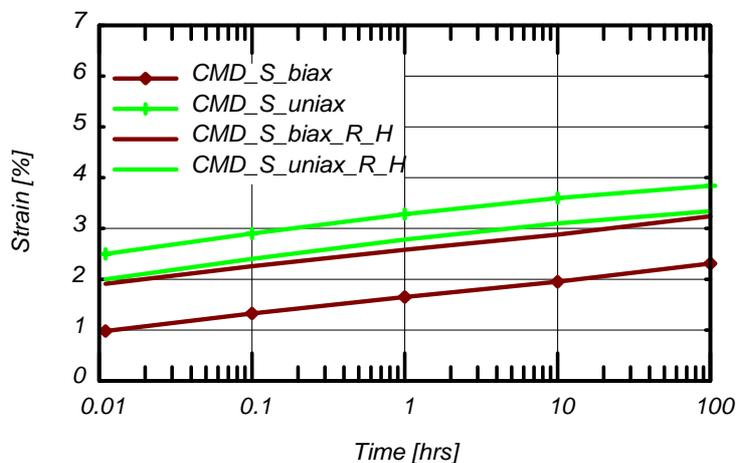
**Figure 11.** Sustained loading tests at University of Strathclyde, Modification with Ramp – Hold, CMD, grid type B
