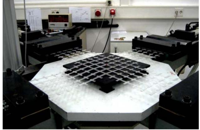
**Figure 5.** Biaxial testing equipment at University of Essen
