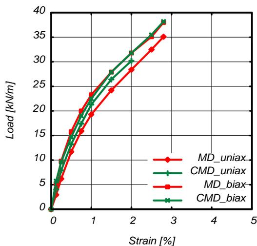
**Figure 8.** Stress-Strain Curves for Uni- and biaxial CRS testing Kupec (2004) and McGown *et al.* (2004)
