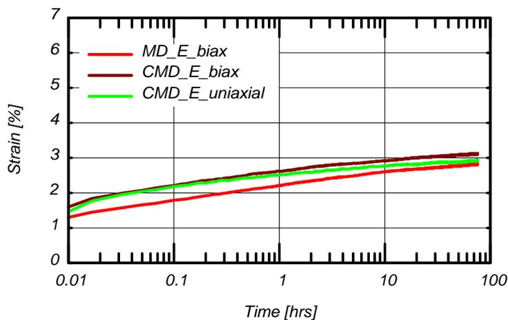
**Figure 10.** Sustained loading tests at University of Essen, grid type B
