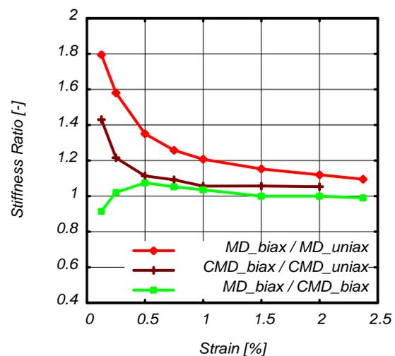
**Figure 9.** Stiffness ratio for MD and CMD derived from CRS testing at Univ. of Strathclyde, see Figure 8
