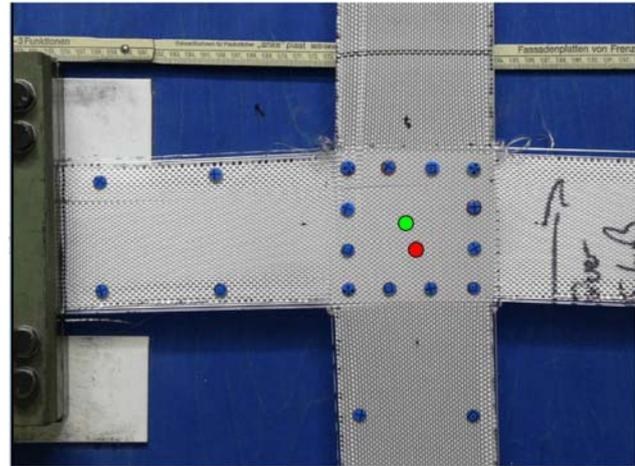
**Figure 3.** Biaxial testing of a woven geotextile at RWTH Aachen, situation just before break
