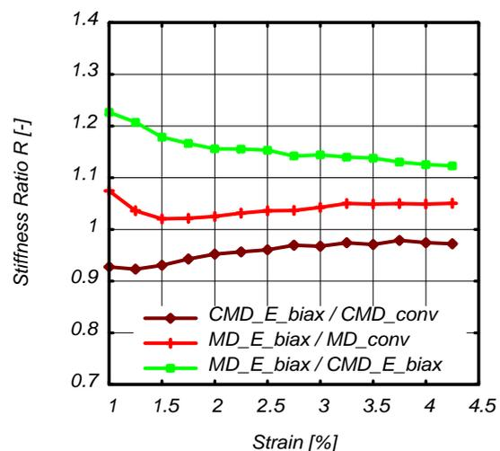
**Figure 7.** Stiffness ratio for MD and CMD derived from CRS testing at Univ. of Essen (bi\_ax. & uni\_ax.) and conventional wide-width testing (DIN EN ISO 10319), stiffness variation of MD and CMD
