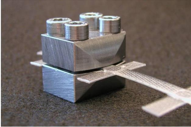
**Figure 4.** Single strip clamping of geogrid developed for biaxial testing at University of Essen
