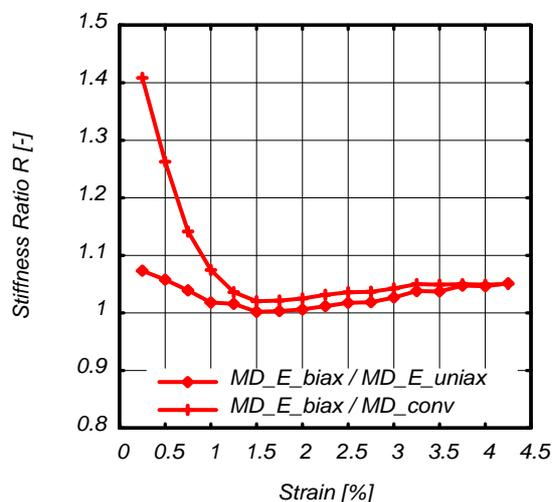
**Figure 6.** Stiffness ratio for MD derived from CRS testing at Univ. of Essen (bi\_ax. & uni\_ax.) and conventional wide-width testing (DIN EN ISO 10319)
