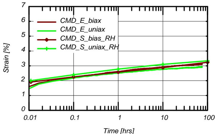
**Figure 12.** Sustained loading tests at University of Strathclyde, Modification with Ramp – Hold, and University of Essen, CMD, grid type B
