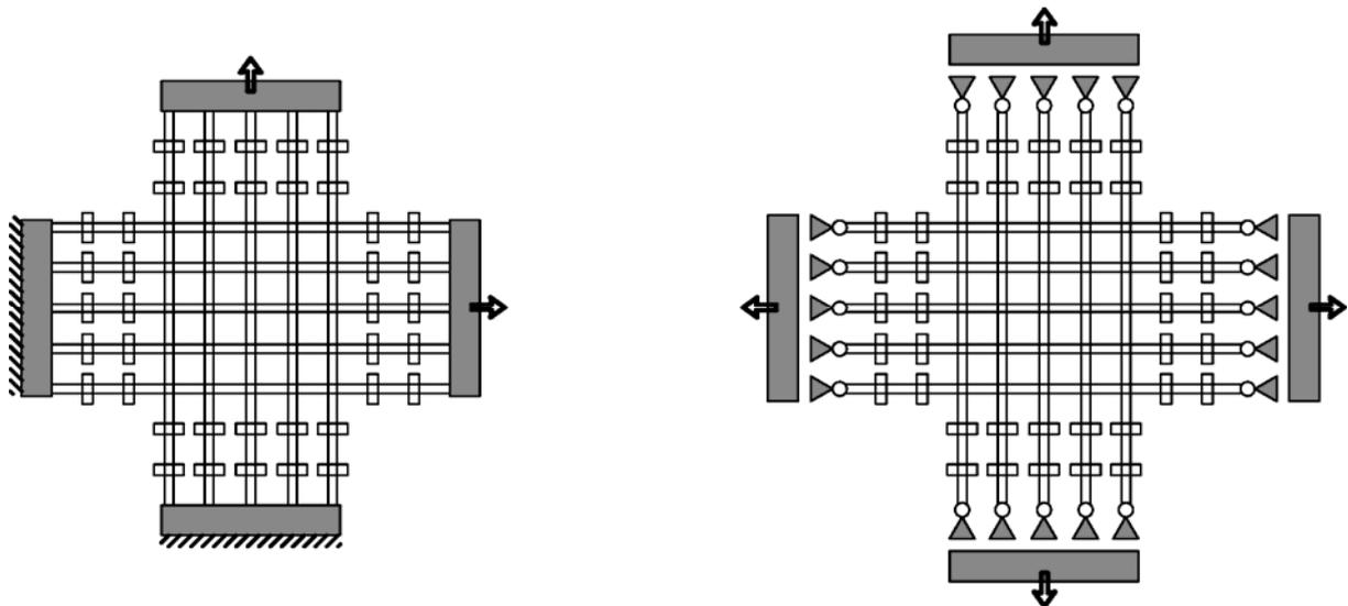
**Figure 1.** Left: inadequate loading arrangement (equipment at University of Strathclyde now RWTH-Aachen, McGown *et al.* (2004); Right: improved biaxial loading (equipment at University of Duisburg / Essen)
