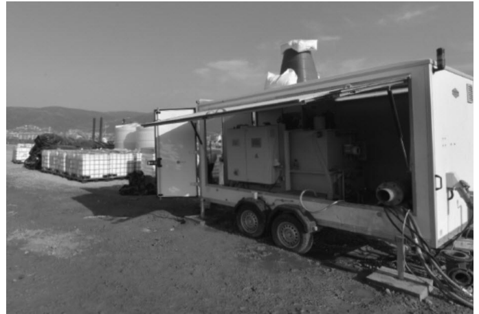
Figure 2. Example of mobile dosing unit for addition of flocculation agent into tailings flow (Courtesy of Clariant)
