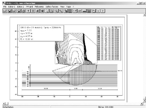
Figure 4 Example of stability analyses results.
