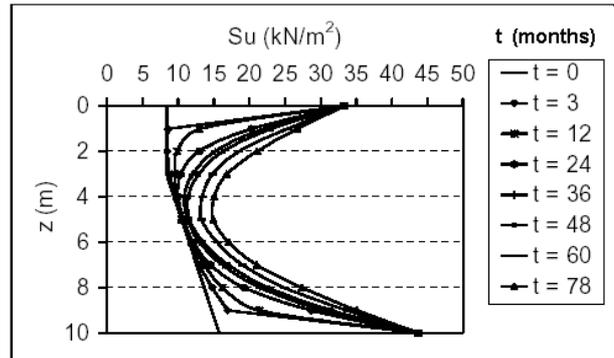
Figure 3 Example of the undrained strength of the soil foundation evolution in zone 1.
