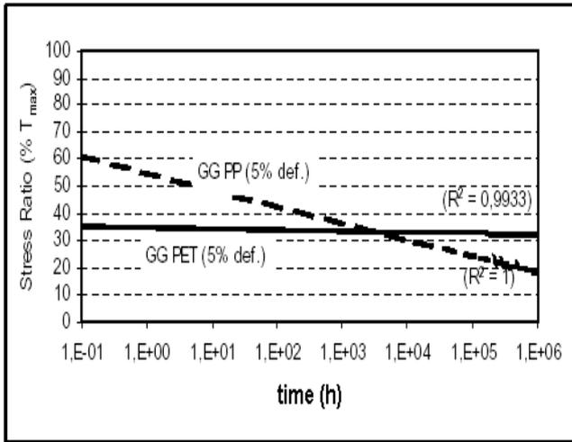
Figure 8 Tensile strength at 5% of deformation (creep tests) (BBA 1999).
