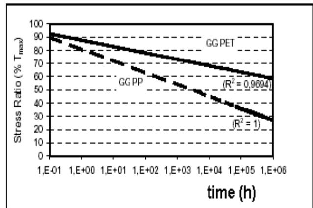
Figure 7 Rupture behaviour of the considered geogrids (BBA 1999).
