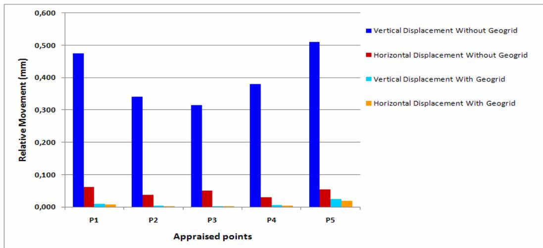
Figure 7. Maximum relative displacements measured in each case: vertical and horizontal relative movements of crack walls on areas with and without geogrid.
