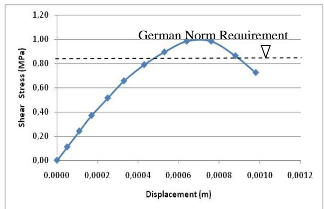
Figure 11. Direct shear test result.
